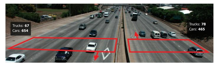
IQ-110, as part of IQ-InfinityTM, will count and give a cumulative total of the number of objects that have passed through one or more areas of interest that are drawn on the screen. The software will count traffic that passes through a region in specified directions whilst ignoring traffic from other directions. Sophisticated filters, including human templates, and the ability to see perspective can be used to ignore unwanted objects and focus only on humans or cars for instance.
